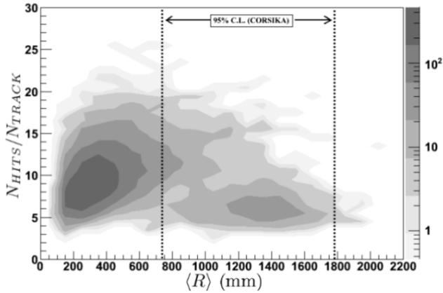
**Fig. 4.** The recorded multi-track events for track multiplicities  $N_{\text{TRACK}} > 4$  displayed according to the bundle size and reconstruction purity ( $\langle R \rangle$  vs.  $N_{\text{HITS}}/N_{\text{TRACK}}$ ). The number of events is indicated by contrast and the dashed lines indicate the limits of CORSIKA-expectation (the region of 95% of air showers).
