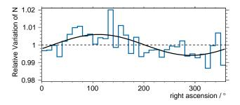
**Fig. 2.** Relative variation of the event rate in right ascension due to the weather effect. We plot the quotient of the event rate of the data set subject to an energy cut (1 < E / EeV < 2) with and without applying the energy correction. The sine fit performed to guide the eye and estimate the effect on first harmonic modulation studies yields an amplitude of ~ 0.6%. This amplitude estimate ranges from 0.2% to 1.5% at all relevant energies.
