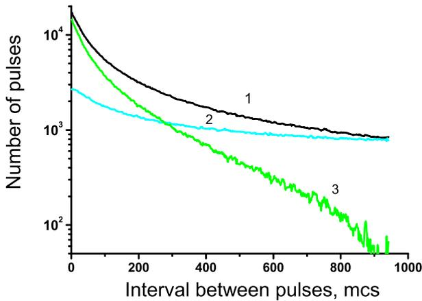
**Fig. 2.** Distribution of time intervals between pulses NM in time window  $T_0 = 1000 \mu s$ . 1-for trigger SHAL, 2-for control window, 3-difference between 1 and 2.
