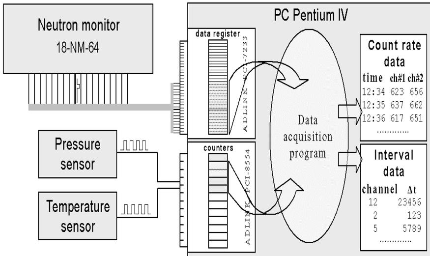
**Fig. 1.** The DAQ of the Baksan neutron monitor.
