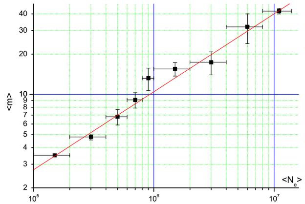
**Fig. 3.** Dependence of multiplicity of neutrons in NM on  $N_e$ .
