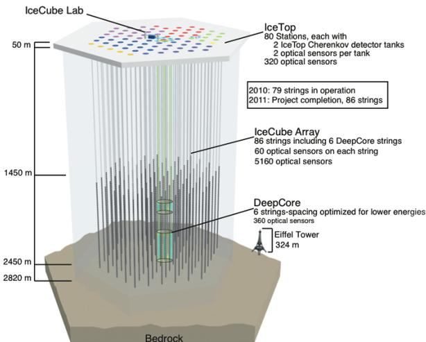
**Fig. 1.** Schematic of the IceCube neutrino observatory.
